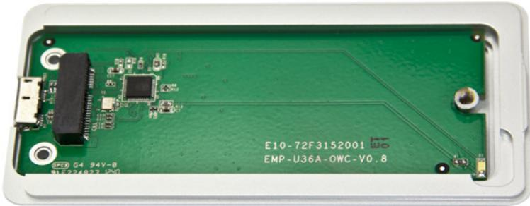
3. Insert the SSD into the black connector (see below-left). The connector is notched so that the SSD fits using only one orientation. Next, use the short Torx T5 screw to hold the SSD in place (circled below-right). Do not over-tighten the screw.
