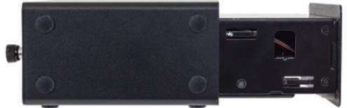
10. Tighten both thumbscrews on the back of the device until you feel resistance. This completes the assembly process. You can now connect the device to power and your host computer with the included cable.
