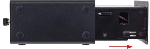
3. Set the outer enclosure aside. Notice there is a fan housing affixed to the inner chassis; this covers the area where SSDs are installed, so it will need to be removed temporarily. Set the inner chassis on your work surface so the fan is facing upward before proceeding to Step 4.
