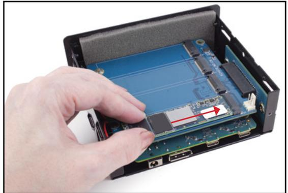
7. Affix each drive's mounting screw as shown. Repeat Steps 6 and 7 for each SSD being installed. The image below-left shows what the device looks like with all four M.2 SSDs installed. Note that you can use different brands and capacities of SSD if you wish.
