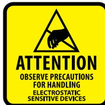
The computer, PCIe card and eGPU are static-sensitive devices. They are susceptible to invisible damage if not protected during installation. We recommend the use of a grounding strap. Make sure to work in a clean, static-free area, and avoid wearing clothing that retains static charges. [www.owcdigital.com/support/anti-static](http://www.owcdigital.com/support/anti-static)
