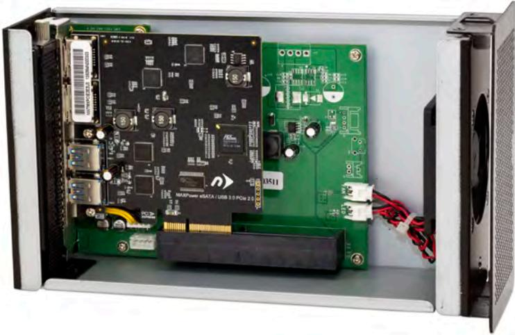
6. Press down on the PCIe card to seat the connectors into the PCIe slot, as shown below. Press straight down; do not twist or rock the card. If the card does not seat fully, do not force it in. Remove the card, check to make sure that there is no damage to the card or the slot and that the bracket is not bent, then try again.
