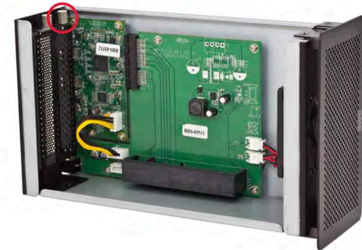
5 Install the PCIe card as shown below. Line up the connectors on the PCIe card with the PCIe slot, and make sure that the edge of the metal bracket on the PCIe card lines up with the slot in the bottom of the Helios.
