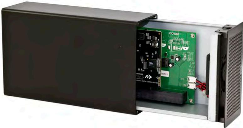
9. When the inner chassis is fully seated into the outer enclosure, tighten the thumbscrews on the rear panel, circled below in red. Press each screw in toward the enclosure, then twist clockwise while still applying pressure. Keep twisting until you feel increased resistance.
