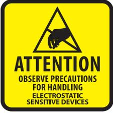
*These are static-sensitive devices. They are susceptible to invisible damage from static electricity if not protected during assembly.*
