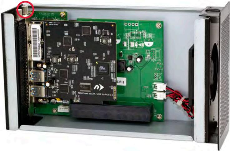
8. Slide the inner chassis back into the outer enclosure as shown below, then turn the Helios so that it is standing on its feet.
