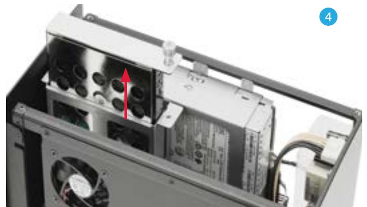
5. Set the drive tray on the work surface as shown.
