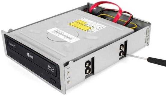
5. Slide the optical drive the rest of the way into the inner chassis, then align the screw holes on the side of the drive with the four screw holes on each side of the inner chassis. Affix the eight included screws with a Phillips screwdriver.
