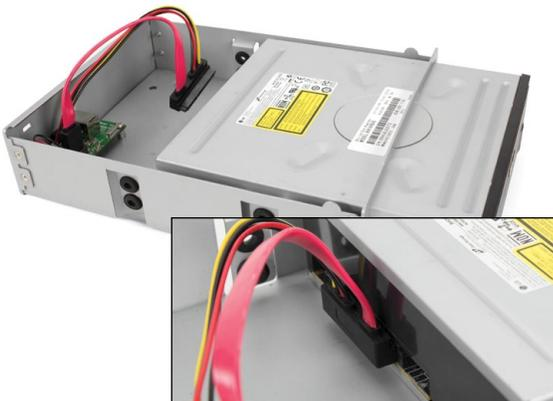
4. Slide the optical drive approximately half way into the inner chassis (left), then connect the SATA power and data cables (below-left).
