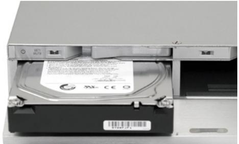
**NOTE:** Be careful to not damage any components — do not force the drives into place. If they do not slide and seat in easily, make sure there are no obstructions.
