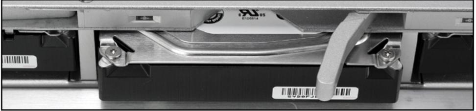
To remove the drive from the enclosure, use the lever located above the drive to eject the drive mechanism (shown above). If more than one drive fails at the same time, or if one drive fails and the RAID mode is set to RAID 0 or Combine (SPAN) mode, the data is lost and the system cannot be accessed again until the drive(s) are replaced and a new array is built. Note that when using a SPAN, only the data stored on the failed drive is lost.
