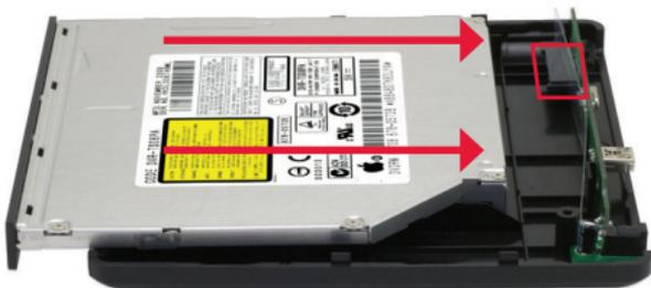
3. Align the edges of the bottom case with the edges of the top cover then slide it forward until the top cover snaps into place.
