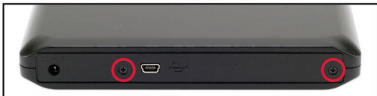
5. Flip the assembled enclosure over and insert the shorter Phillips screw in the location shown. Affix the screw then cover the screw hole with the included rubber foot.
