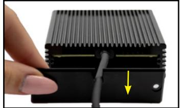
3. Carefully unplug the Thunderbolt 3 cable then connect the approved replacement cable in the same location. Note: this device only accepts Thunderbolt 3 cables with plugs that are 7/8 inch (~ 2.2 cm) long. Other Thunderbolt 3 cable plug types will not fit.
