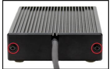
2. Note that the cover has a cut-out on one side; separate the cover from the cable, then set the cover aside.
